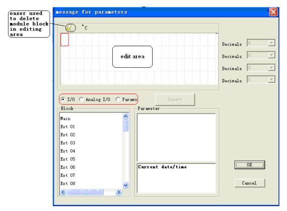
(1) Select "I/O", hereunder "Block" section consists of "Main CPU", 31 pieces expansion modules& SMS module's I/O status blocks, hence any of "Main", "Ext 01", "Ext 02", ... can be selected, as below config shows:
