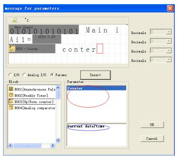
**Notes:** In case the block you would select is just weekly timer or yearly timer under "block" section, then none of parameters can be displayed under "Parameter" section(area circled in red line). However, if you intend to insert system date and time, then you may just select "Current date/time" in area circled in blue line, then click "Insert" button. finally click "ok " button to finish and confirm your insert
