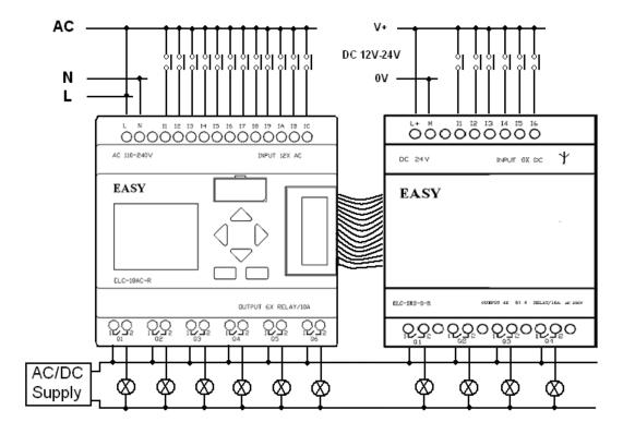
The ELC-SMS-D-R must be connected according to the following schematic:
