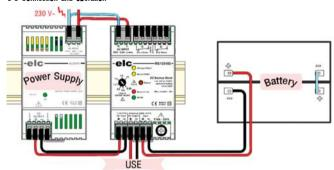
Connect the use in the terminal block "Uninterrupt DC Output". Positive left, negative right.
