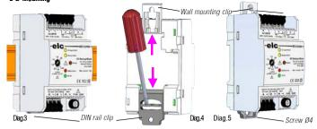
Mounting by CLIP on the profiled 35x15mm or 35x7.5mm (DIN rail EN 50022) :
