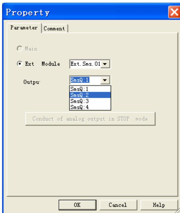
The SMS output used is the same as other modules of xLogic SuperRelay. The ELC-SMS-D-R module is a relay output.
