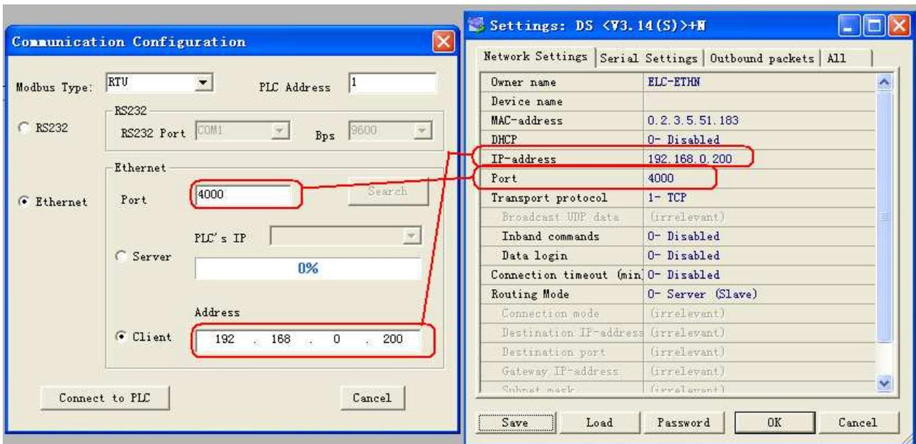
Click "Connect to PLC" button, and then the Ethernet module and PC will be linked.
