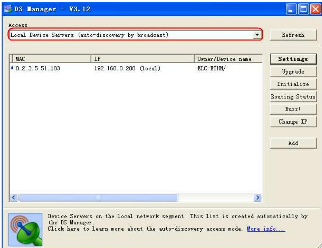
The object module appears as above window shows; it includes "Linking Status", "MAC", "IP", "Owner/Device name"
